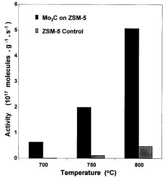
**Figure 2.** Catalytic activity for dehydroaromatization of methane by sonochemically prepared Mo<sub>2</sub>C/ZSM-5 and sonicated ZSM-5 control.
