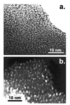
**Figure 1.** STEM micrographs of Mo<sub>2</sub>C/ZSM-5 prepared sonochemically showing (a) the lattice fringes of the ZSM-5 and (b) a typical dark field image showing Mo<sub>2</sub>C particles on the surface of the ZSM-5.
